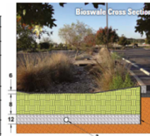
A bioswale captures, conveys, and filters runoff at the Dim Rural Center. Lateral hydraulic restriction barriers protect the adjacent pavement subgrade while allowing natural infiltration.
