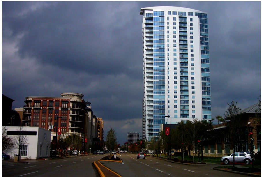
The more-than-30-story building on the right has a significantly lower per capita imperviousness than the seven-story building on the left, but the seven-story building has a much better return on investment in terms of the environmental benefits received. The additional 20+ stories provide only marginal improvements in runoff quality versus the shorter building (see Figures 4 and 5).
