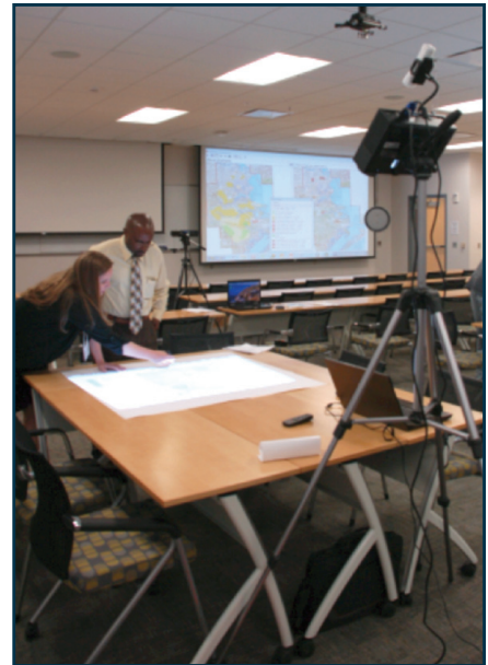
Figure 1: A weTable setup- the Wiimote device is atop the projector. The image is cast onto the table.
