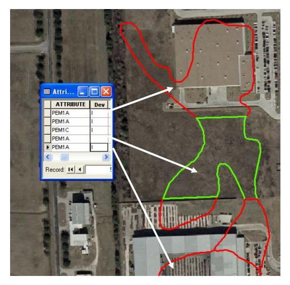
**Figure 4. Wetland polygon from NWI overlain on 2002 color photo.** Developed area is cut out and reclassified as "I", which stands for "Industrial/Commercial" in the attribute table. The undeveloped area is left blank in the new field for 2002 status. A query method allows the "change" in 1990 habitats to be calculated.
