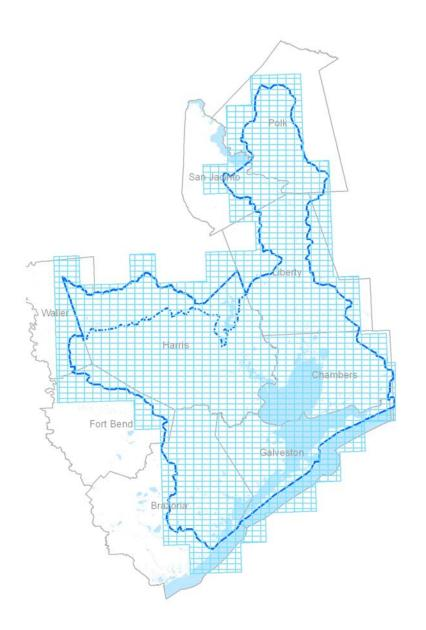
Figure 5 – Lambert grid used to create relative wetland loss map
