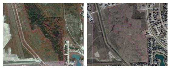
Figure 8.1995 photo on left shows NWI polygons which have been filled by 2002 photo on the right. Note that the wetland photographic signature has completely disappeared on the 2002 photo, but no obvious development has taken place.
